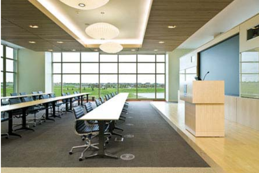
Conference room at the LEED Platinum Great River Energy building in Maple Grove, Minn. Note the underfloor air diffusers in the floor and high windows for daylighting.
